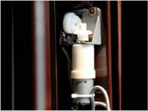
SCROCCO ELETTRICO ELECTRIC DEVICE FOR REMOTE OPENING
